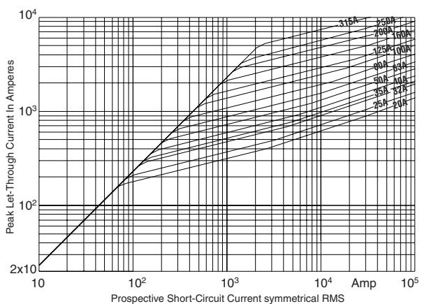
\* 315 amp fuse is derated to 900V
