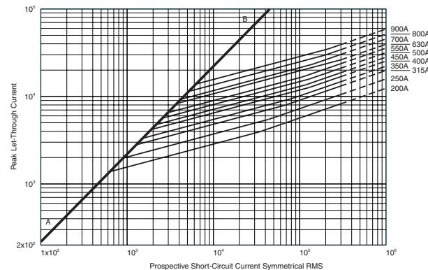
900 amp fuse is derated to 550V (IEC).
