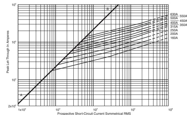
630 amp fuse is derated to 1100V (IEC).
